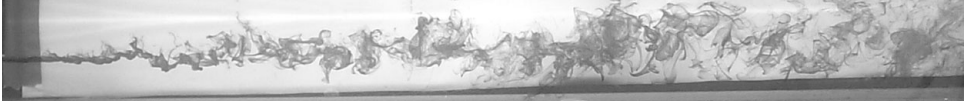
FIGURE 1. Dye visualization of the plume at Re = 10\,000 with a nozzle diameter of D_{nozzle} = 4.7 mm.
